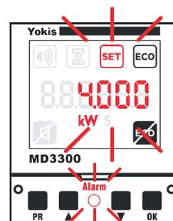
❗ The transmission of commands to radio receivers is shown by the lighting of the icon **🔊** on the device display.
