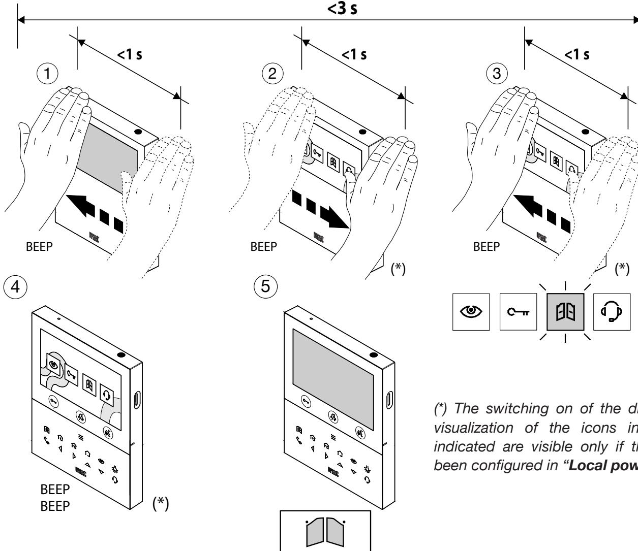
(\*) The switching on of the display and the visualization of the icons in the screens indicated are visible only if the device has been configured in "**Local power**" mode.
