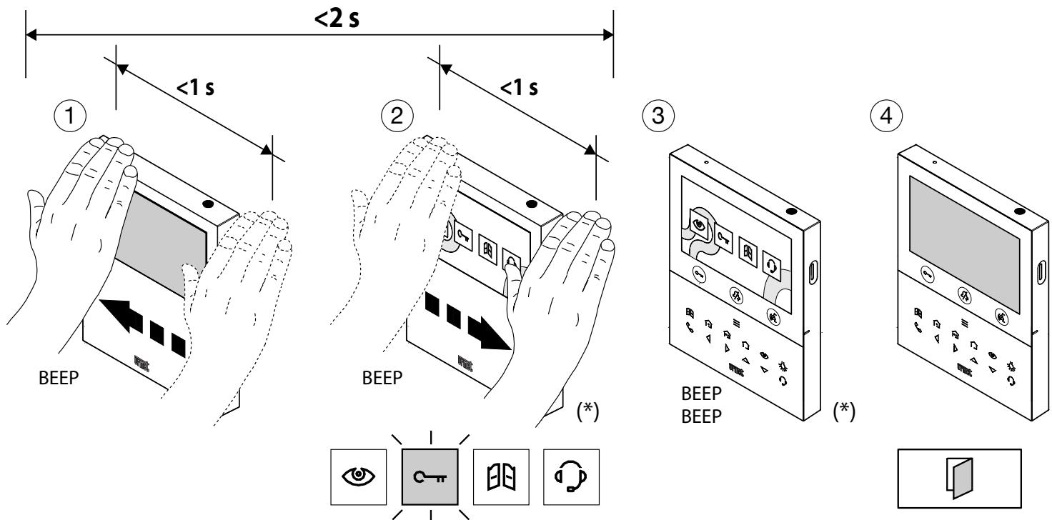
(\*) The switching on of the display and the visualization of the icons in the screens indicated are visible only if the device has been configured in “***Local power***” mode.
