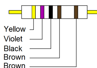
Colour code for resistor 4.7 kohm, tolerance 1%
