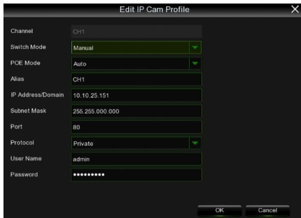
To modify the connected cameras' Network Settings (e.g. to modify the camera IP address from DHCP to Static, Subnet Mask, Gateway, Port) select (see the circles in previous picture).
