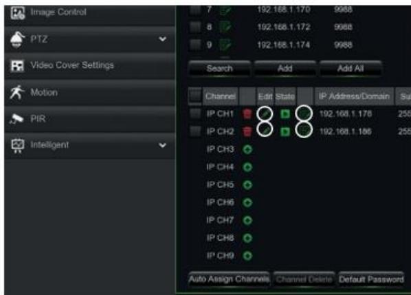
It is possible to modify the parameters used by the HVR to establish the connection to each added channel selecting the button (see the circles in previous picture).
